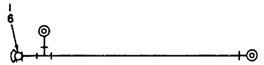
HYD PUMP AIR LINE HOSE (LOOSE STORE IN FRONT PUMPS)
